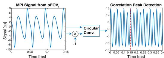
**Figure 1:** Phase shift estimation for one partial field-of-view.
