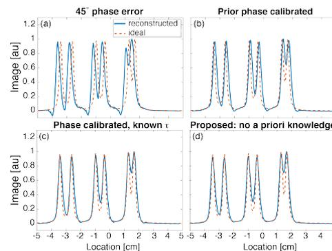
**Figure 3:** Comparison of the proposed method with calibration-based techniques. In each plots, dashed line is the ideal image without relaxation, solid line is the reconstructed MPI image.
